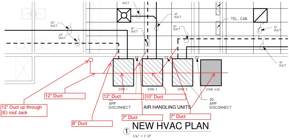
Provide new Outside Air duct from existing roof ventilator, connect to return air trunk line. Provide volume dampers at each unit.
