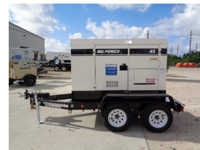
Example of a 50 b.h.p. generator.
