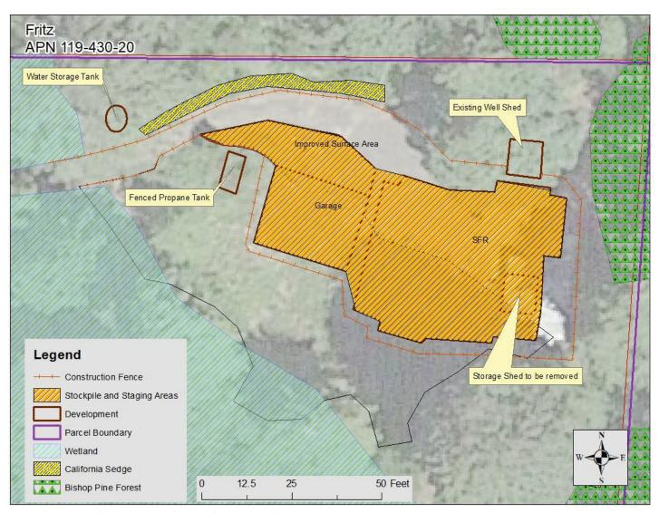
Figure 3. Locations for construction fence, and stockpile and staging area.
