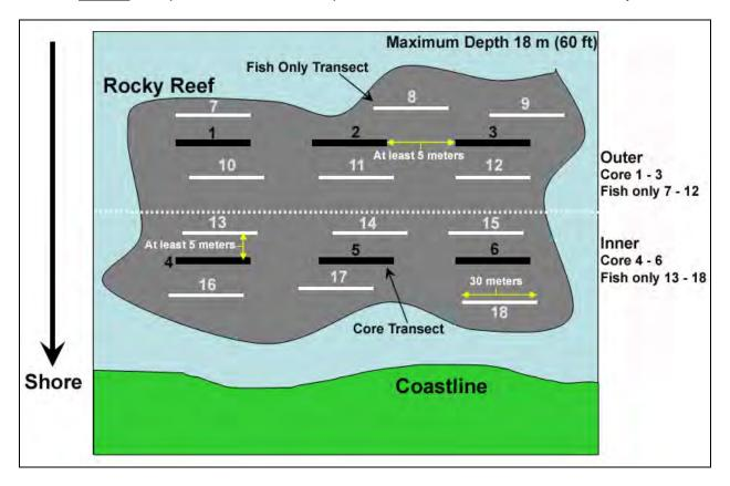
Figure 9. Diagram of transects over a rocky reef. All teams should aim to complete six core transects, which are marked in bold (3 in each zone), plus an additional twelve random fish only transects, which are marked in white (6 in each zone). All transects are 30 meters in length.
