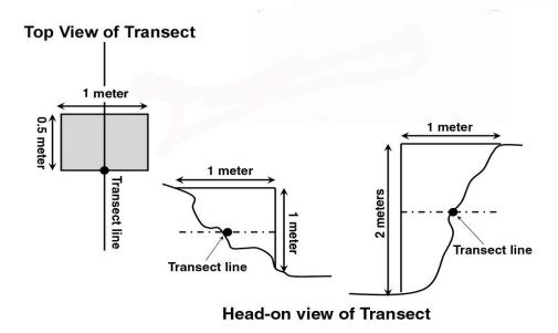
Figure 18. Physical relief is measured as the greatest vertical relief within a 1-meter wide section across the tape and .5-meter section in front of each point
